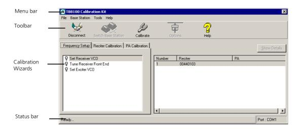
The main program window has three tabs. The Calibration Wizards displayed on each tab are only visible once you are connected to the reciter and/or base station.
